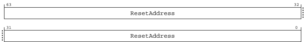
Figure A-165: AARCH64_RVBAR_EL2 bit assignments
